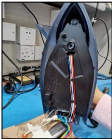
Open-up to access the cable at the Bottom of Tank
