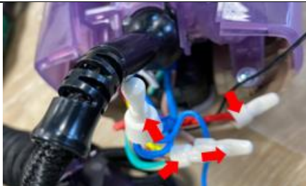
Connect all Wires, assemble CLOSED END CONNECTOR 16 & 17 per instruction in page 15
